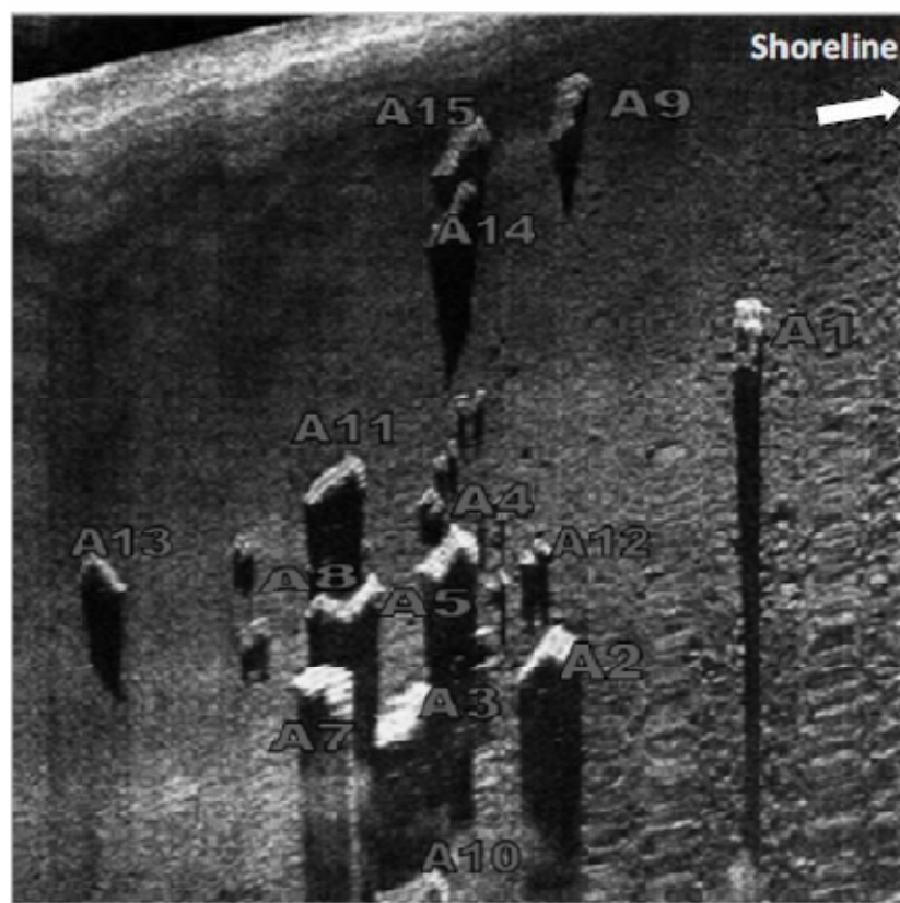
Figure 4: Side Scan Imaging showing the position and location of WABCORE blocks
