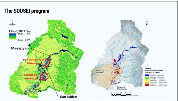
Figure 7.3.2 Results from inundation analysis of the Pampanga river basin by using the RRI model. Map ©ICHARM
