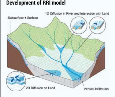
To predict the behavior of largescale inundation in low-lying areas in a short period of time, ICHARM has been developing a new numerical model called Rainfall-Runoff-Inundation (RRI) model. The model simulates various hydrologic processes including rainfall-runoff, streamflow discharge, and inundation over floodplains in an integrated manner.
