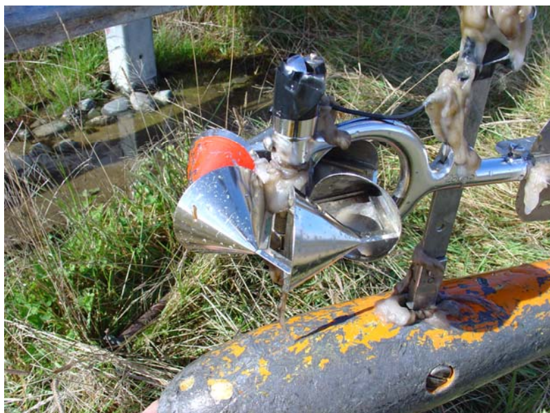
Figure 1 Shows didymo mat around spindle of Gurley type current meter and hanger bar following an attempted river flow gauging of the Mararoa River.
