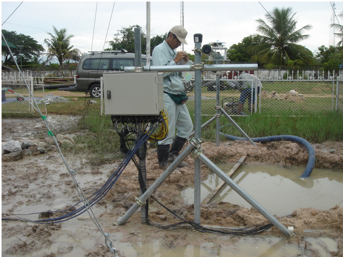
Picture A: Soil moisture sencer connected with data logger with AWS
