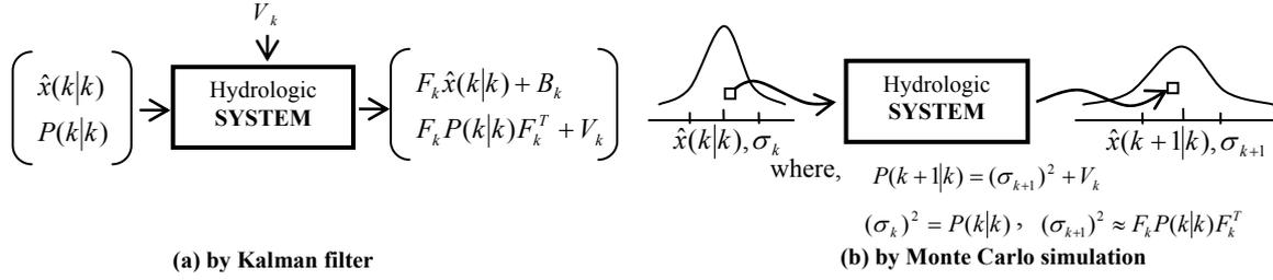
**Figure 5.** Time update algorithm of the Kalman filter
