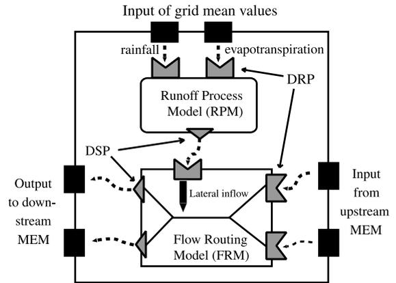
Fig. 4. Structure of the MaScOD element model (MEM).
