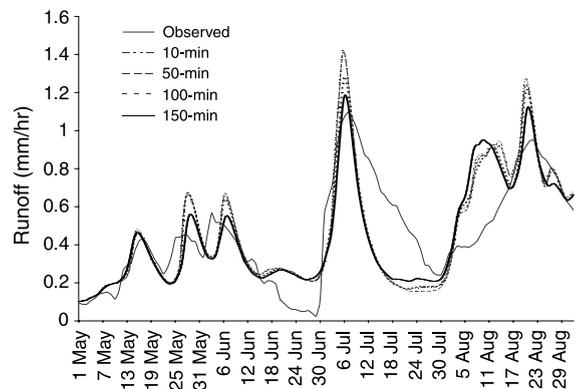
Fig. 8. Simulated hydrographs at Bengbu (132,350 km<sup>2</sup>) obtained from various input data resolutions.
