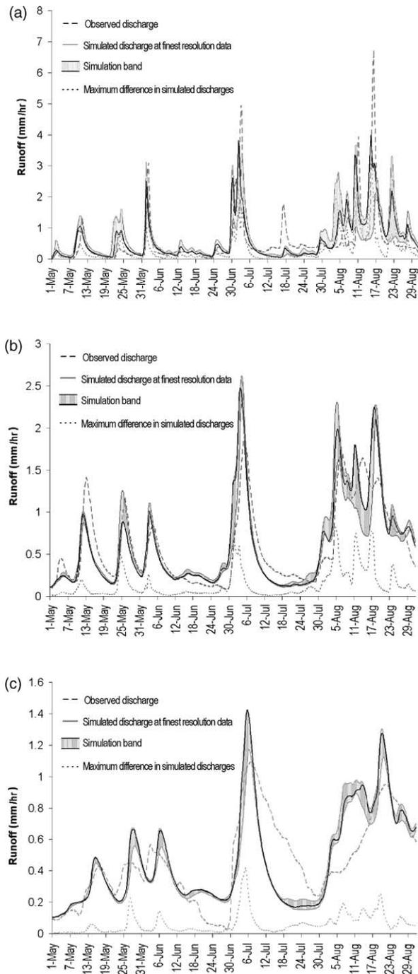
Fig. 9. The simulation band for hydrographs at (a) Suiping (2093 km<sup>2</sup>), (b) Wangjiaba (29,844 km<sup>2</sup>), and (c) Bengbu (132,350 km<sup>2</sup>) produced by overlapping the hydrographs obtained from different resolutions of input data yields. It can be seen that the finest resolution data is not necessarily the best.
