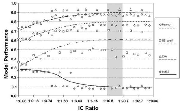
Fig. 13. Model performance versus IC-ratio for four indices.
