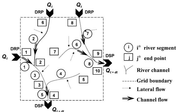
Fig. 3. Schematic of the flow routing model (FRM).
