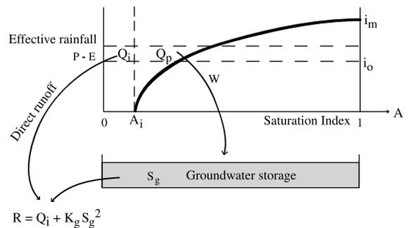
Fig. 2. Schematic of the runoff process model (RPM).
