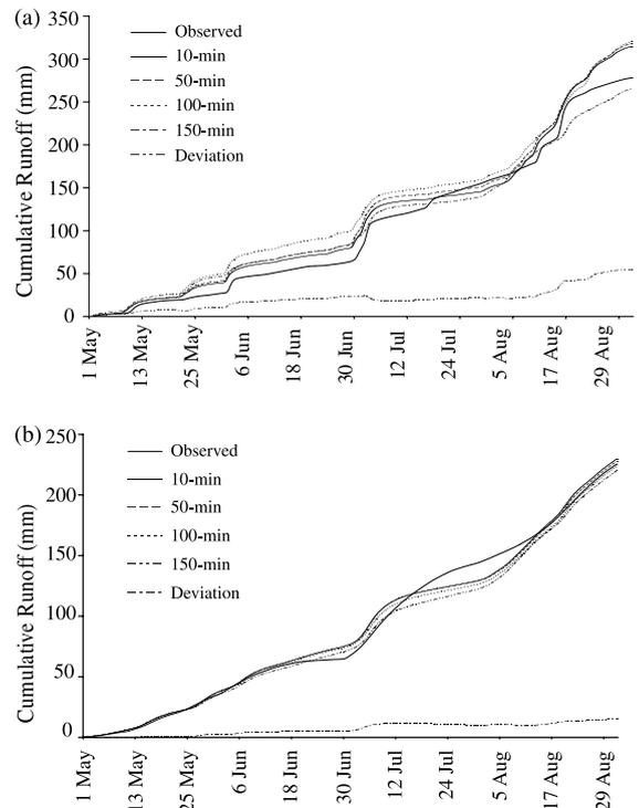
Fig. 10. Cumulative runoff for various input data resolutions (a) at Suiping (2093 km<sup>2</sup>) (b) at Bengbu (132,350 km<sup>2</sup>); the smaller catchment has the larger difference in accumulated discharge.
