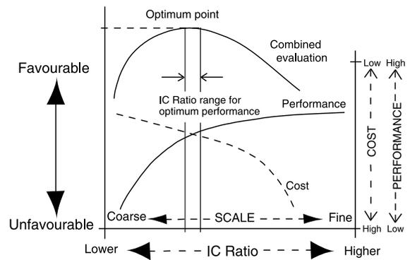
Fig. 14. Trade-off between model performance and model cost with respect to scale in terms of the IC-ratio.
