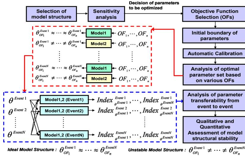
**Fig.1** Schematic illustration of a framework to assess model structural stability;  $\theta_i^j$  = optimal parameter set;  $Index_k^j$  = measurement value for assessment of parameter transferability;  $i$  = Objective Function;  $j$  = storm event;  $k$  = optimal parameter set of each event.
