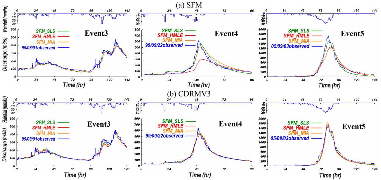
**Fig.3** Comparison between the simulated and the observed hydrographs according to three objective functions; (a) SFM cases, (b) CDRMV3 cases.
