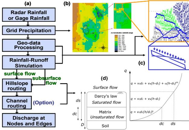
**Fig.2** Schematic representation of CDRMV3 (a) Modular structure of CDRMV3 (b) Distributed grid rainfall data (c) Slope and channel components extracted from DEM (d) Model structure for the hillslope soil layer and discharge-stage relationship.
