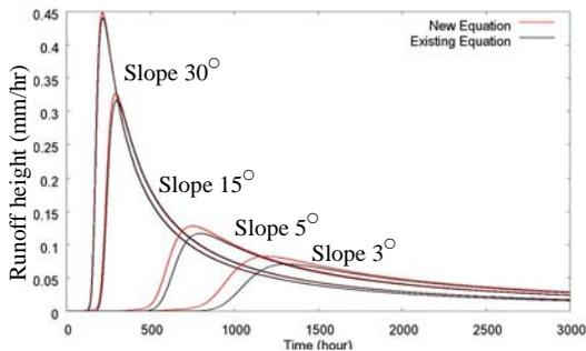
**Fig. 9** Test case 2 – Simulated hydrographs for different slope angles.
