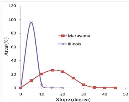
**Fig. 3** Slope-area comparison for the Maruyama and the Illinois River basins.
