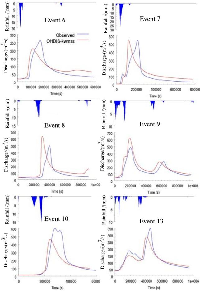
**Fig. 2** Model calibration and validation at the Illinois River basin.
