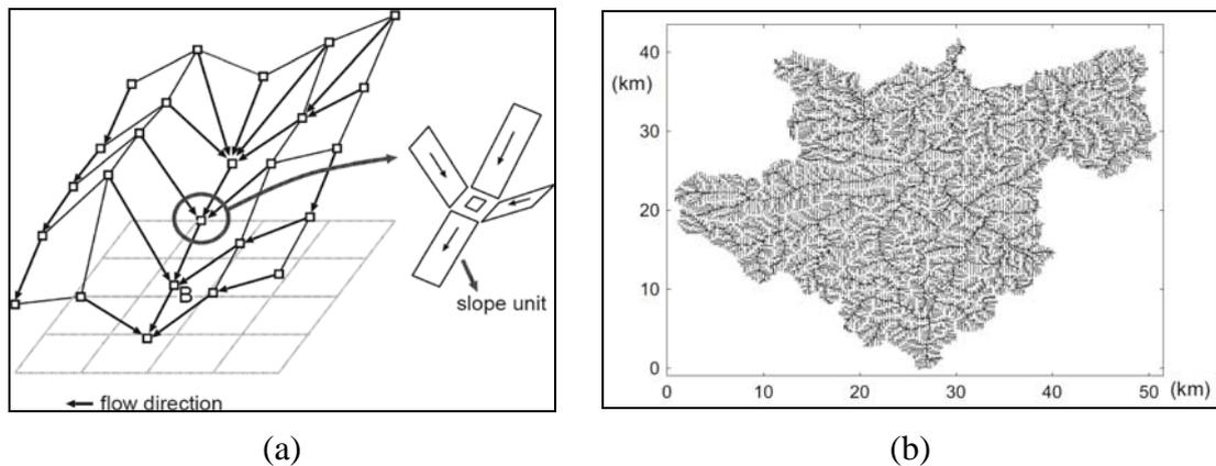
**Figure 2: Schematic drawing of a watershed model using the 8-direction method (a) and an example of flow direction information derived from DEM (b)**
