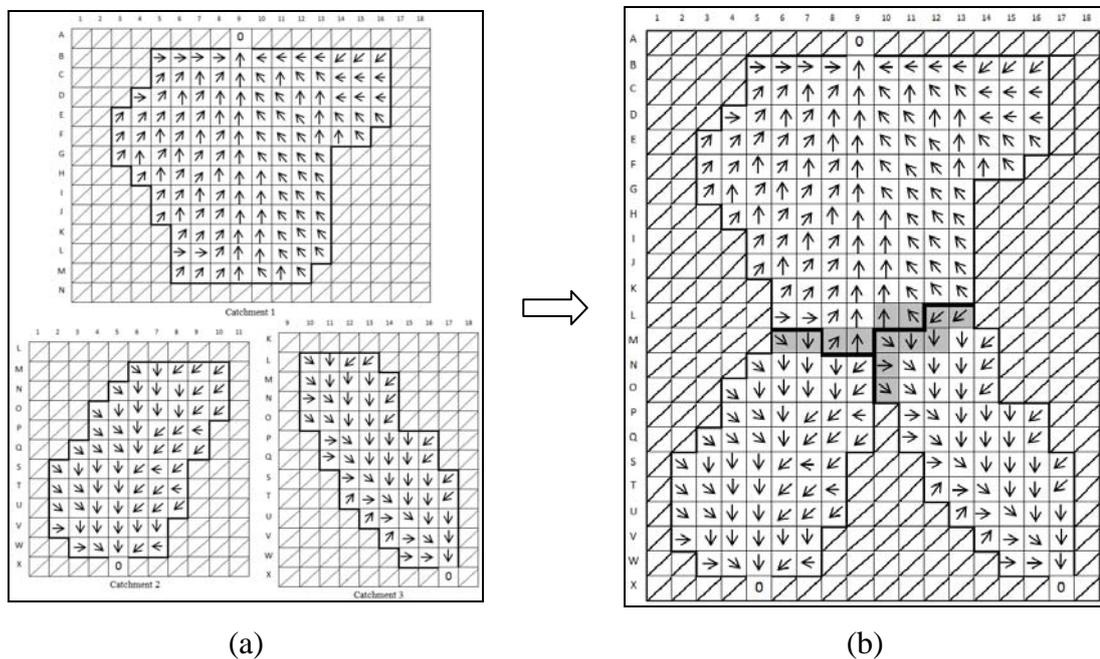
**Figure 1: An example of flow direction data before (a) and after joining (b) (Arrows: flow direction; gray cells: overlapped cells; bold lines: basin divides)**
