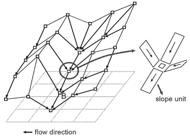
Fig.2 Schematic drawing of a watershed model using the 8-direction method.
