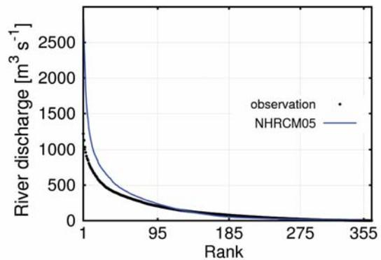
Fig. 4. Flow Duration Curve of 20-years-mean river discharge. Black dots show the observed inflow in Bhumibol Dam and blue line shows the simulated result using NHRCM 5km forcing data.
