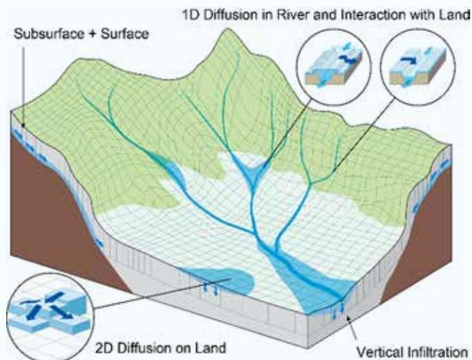
To predict the behavior of large-scale inundation in low-lying areas in a short period of time, ICHARM has been developing a new numerical model called Rainfall-Runoff-Inundation (RRI) model. The model simulates various hydrologic processes including rainfall-runoff, stream-flow discharge, and inundation over floodplains in an integrated manner.
