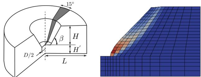
Fig.: Stability analysis of excavation
