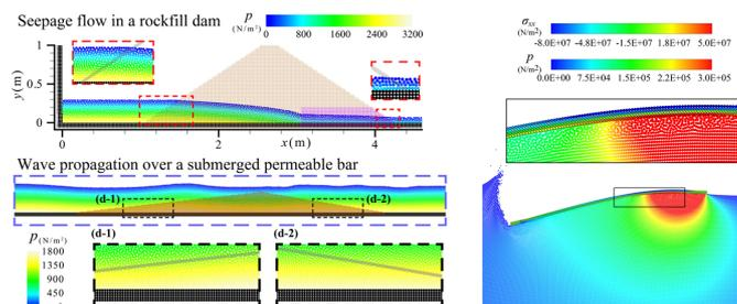
Fig.: Multi-physics simulations by particle methods (FPI and FSI)
