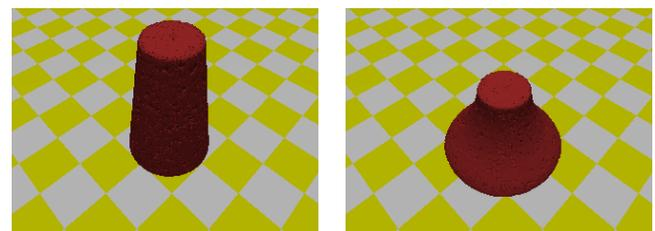
Fig.: Simulation of concrete slump test
