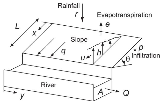
**Fig. 1.8:** Flow modeling using the kinematic wave model.
