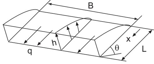
Fig. 3.1: Shallow water flow on a rectangular plane.
