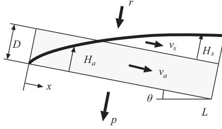
**Fig. 3.3:** Kinematic wave model integrating surface-subsurface flow.
