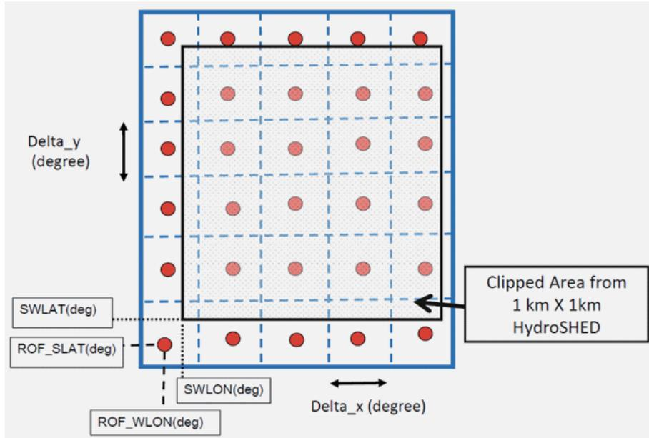
Fig. 4.8: Coordinate system of the rainfall input data.
