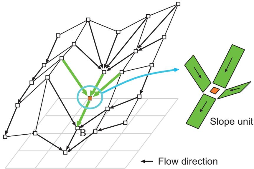
**Fig. 1.7:** Slope element based on flow information.
