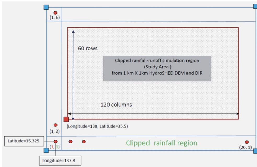
**Fig. 4.9:** Relation between the basin topography coordinate system and the rainfall coordinate system.
