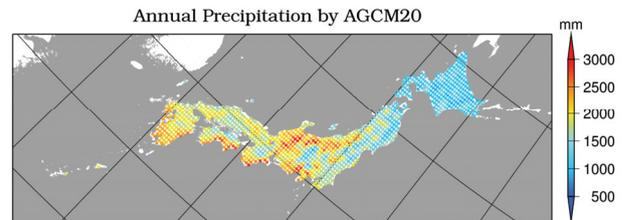
**Fig. 1(b)** Annual mean precipitation from the controlled run output (1975~2003) of the AGCM20. It shows 0.78 of spatial pattern correlation to the observation, and the mean annual precipitation is 1703.8mm.
