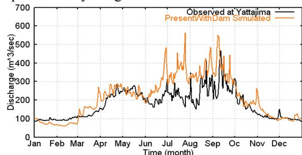
**Fig. 10** Observed river discharge (25 years average) at the Yattajima st. of the Tone River and simulated discharge using the AGCM20 controlled run output
