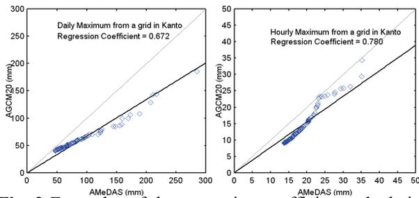
**Fig. 2** Examples of the regression coefficient calculation with the daily and hourly maximum precipitation values of the AGCM20 output and the AMeDAS.
