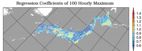
**Fig. 3(b)** Regression coefficient of 100 hourly maximum precipitations from the AGCM20 controlled run output to the AMeDAS observed one.
